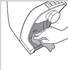
**8** Wipe the inner compartment with a damp cloth and then with a dry cloth.
