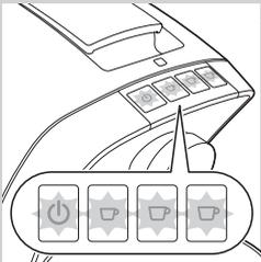
*Note: If after the rinsing cycle the orange service indicator light continues to flash and the yellow lungo button lights up continuously, repeat steps 13-17 once more and make sure the water tank is filled up to the MAX indication.*
