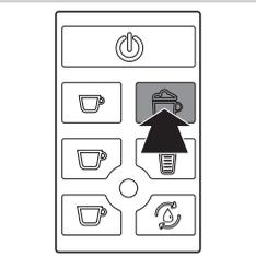
**When the machine has finished brewing the café latte, the orange rinse milk circuit button lights up to indicate that the milk circuit must be rinsed. See section 'Rinsing the milk circuit'.**
